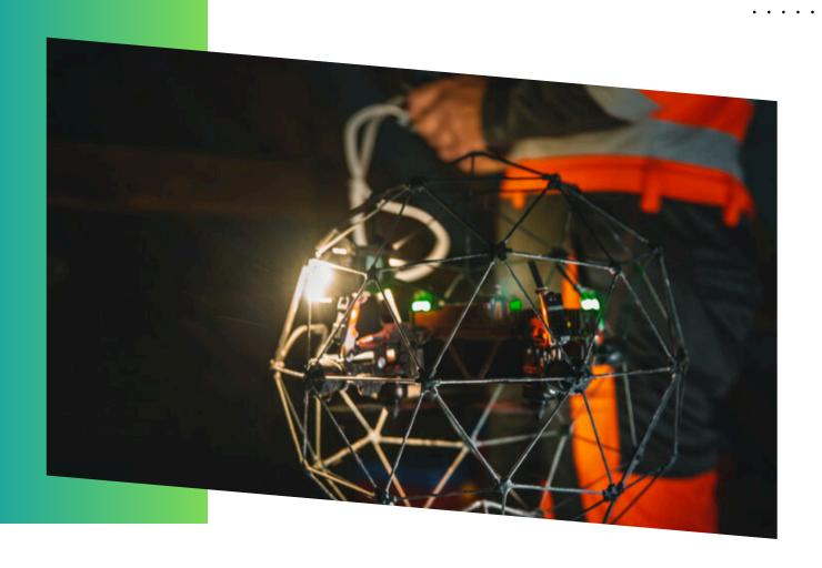
Our drone solutions revolutionize confined space inspections by safely accessing challenging, high-risk environments without the need for human entry. Equipped with specialized cameras and sensors, drones capture critical data inside tanks, silos, vents, and pipes, identifying structural defects, corrosion, or hazardous conditions.
